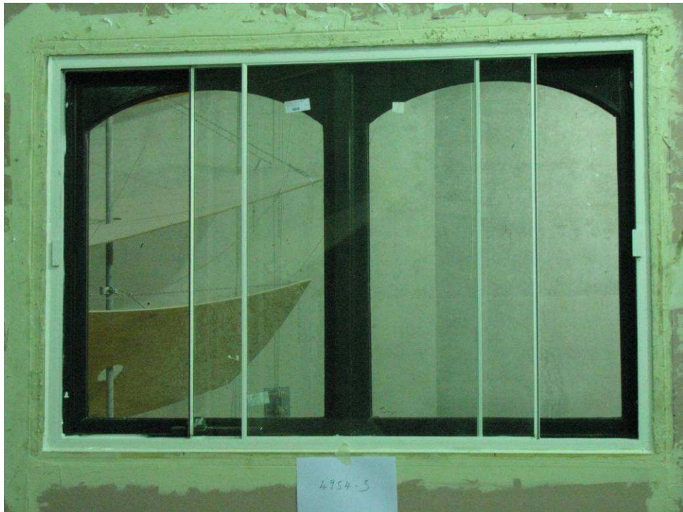
Figure 2. Installation of combined Secondary Window System with 507/508 Ultra Slim Sliding Window open
